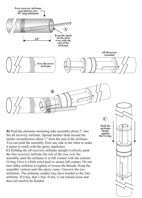
NOTE: In this step you will be using the free end of the straps that you mounted to the fore and aft recovery assemblies.
