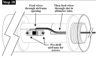
Feed the wire ends into the airframe opening, then through the slot in the altimeter tube and finally out through the end of the altimeter tube. Set the switch into the airframe hole (or stand-off), pre-drill the airframe for the mounting screws, and install the screws. Mark the airframe near the switch for the on-off positions.
