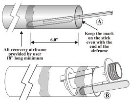
B) Push the altimeter mounting tube assembly about 2" into the aft recovery airframe. Spread another bead around the inside circumference about 1/2" from the end of the airframe. You can push the assembly from one side to the other to make it easier to reach with the epoxy applicator.
