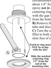
A) Spread a layer of epoxy around the circumference of the opposite end of the tube about 1/4" from the end. Leave a 1" gap in the epoxy not in line with the slot. Push the notched centering ring onto the tube with the notch aligned with the gap in the epoxy. Position the ring 1/2" from the bottom. Allow the epoxy to cure.
