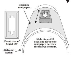
Simply drape a piece of medium sandpaper over the airframe and hold it in place with one hand. Holding the stand-off with your other hand, move the stand-off back and forth along the sandpaper until the back of the stand-off has the desired contour.
